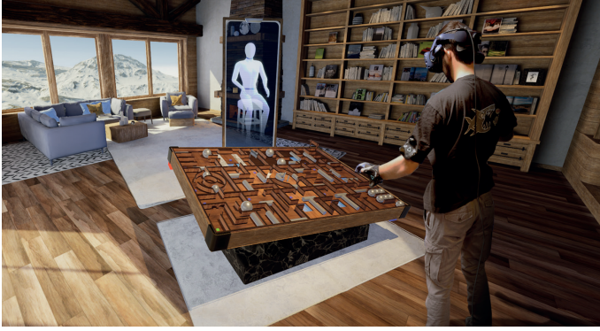
Figure 1. User with the headset, and sensors strapped to his upper limbs and waist, solving a maze in VR using his shoulder's movements as input. On the screen in the background, a holographic coach stands ready to re-explain the motor tasks or to correct the user in case of erroneous movements. See also a demo video available at https://youtu.be/BACpVS4HW40?si=3lIaql9EZ224Umw .
